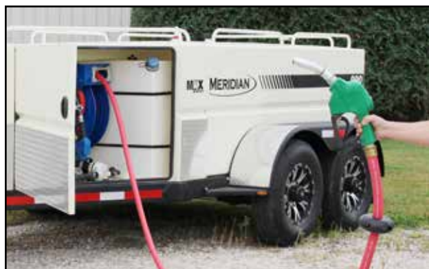
Fig 37 - Hose with green nozzle is for diesel fuel
