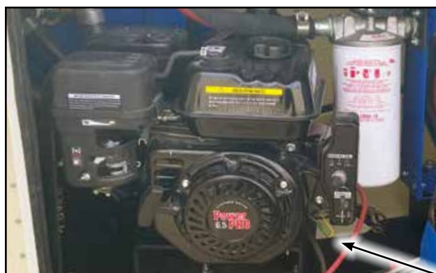
Fig 2 - Engine serial number located behind key switch
