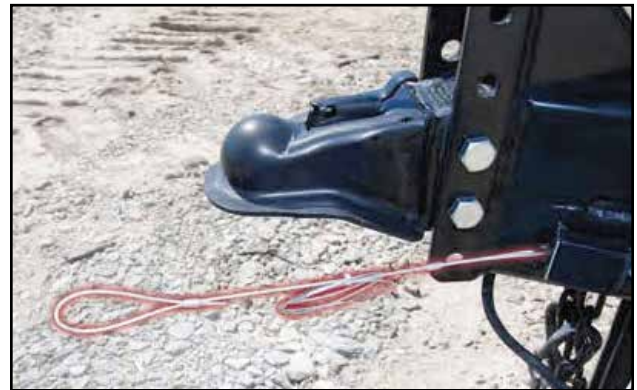
Fig 59 - Break-Away switch and pin
