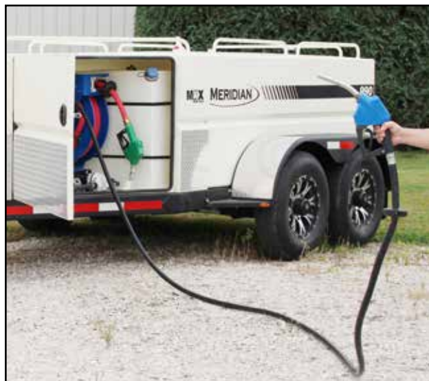
Fig 52 - Hose with blue nozzle DEF fluid
